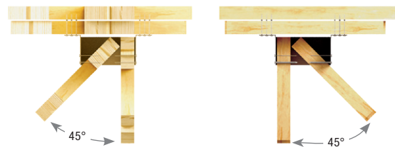
Typical HJC/HTHJ installation top view
